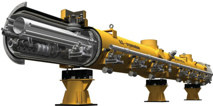
Fig. 10.11 Cut-view of the cross section of ILC cryomodule. Cavity and other components are seen in the picture (© Rey.Hori/KEK)
