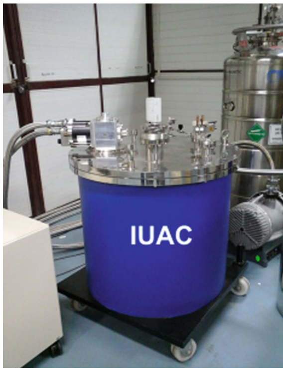
Fig. 9.31 Photograph of the complete CFSM system with central 50 mm RT bore and all feed-thrus (Courtesy IUAC, New Delhi)
