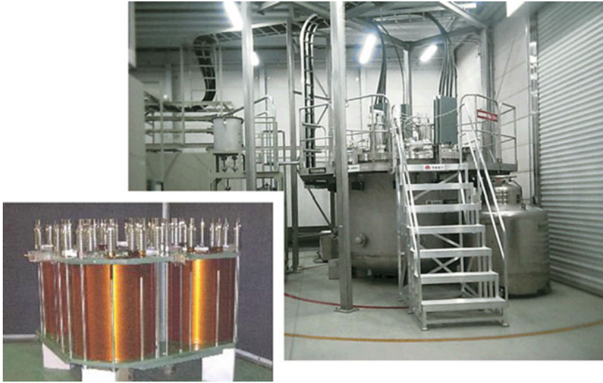
Fig. 12.27 5 MVA SMES system with four-pole solenoid design, built by Chubu Electric Power and Toshiba Corp. Power System Co. Japan. The inset on the left are the four-pole superconducting magnet coils [63] (with permission from Elsevier)
