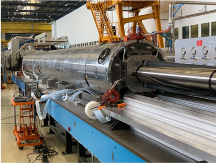
Fig. 10.24 Second prototype 7.15-m-long MQXF-BP2, magnet assembly completed (September 2020) (Courtesy Ezio Todesco, Credit: CERN, high luminosity LHC project and Magnets Superconductors and Cryostat group)
