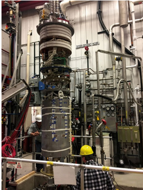
Fig. 10.28 US-MDP ‘Cos \theta – 1’ dipole magnet wound with Nb 3 Sn conductor achieved a field of 14.1 T (4.5 K) at Fermilab in 2019 [43]. Credit Fermi National Accelerator Lab.
