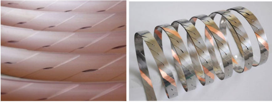
Fig. 6.10 Typical REBCO Roebel cables developed at Karlsruhe Institute of Technology (KIT). Courtesy Wilfried Goldacker, KIT
