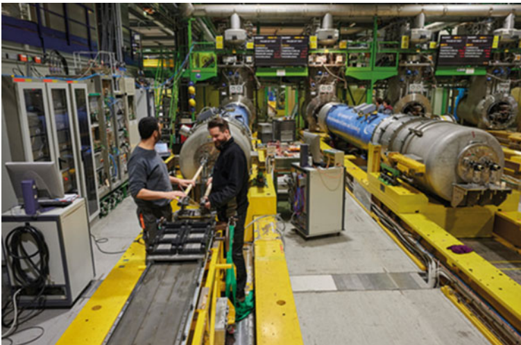
Fig. 10.26 \text{Nb}_3\text{Sn} 11 T dipole magnet for HL-LHC undergoing tests at CERN's SM 18 facility. Credit CERN-Photo-202002-5 [43]
