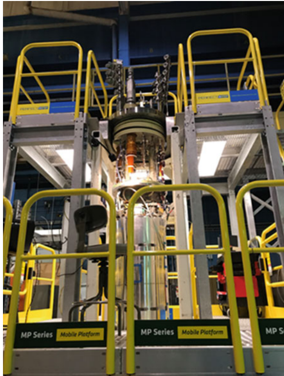
Fig. 10.25 4.2-m-long \text{Nb}_3\text{Sn} quadrupole magnet with 150 mm aperture being readied for test at the BNL, USA [42]. Credit Brookhaven National Laboratory
