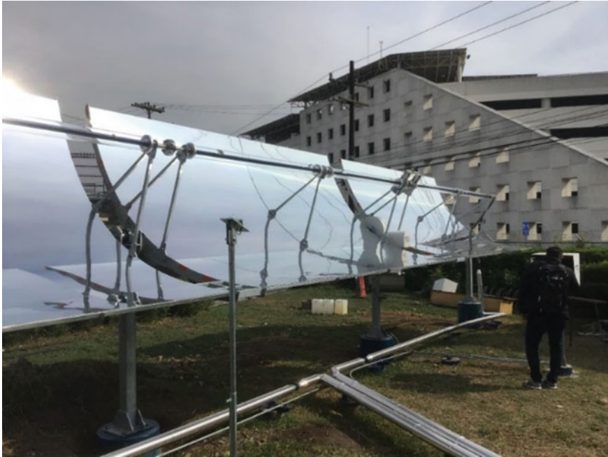
Fig. 19 Parabolic trough solar collector installed in the solar energy laboratory of Tecnológico de Monterrey
