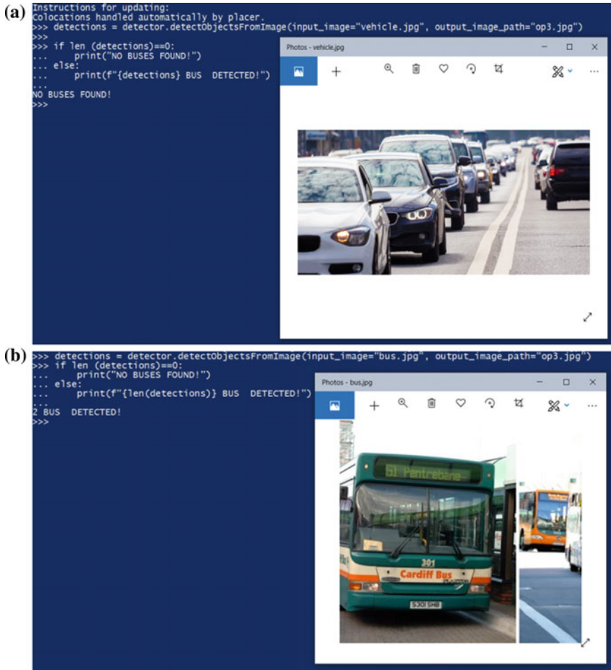
Fig. 9 a Case 1—No buses recognized. b Case 2—Two buses recognized
