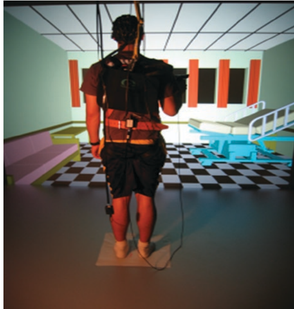
Fig. 3.4 AMTI force platform and 6° of freedoms ultrasound tracking technology from “InterSense, Inc.” was used to control the head and body kinematics and postural responses to visual manipulations of VR scenes
