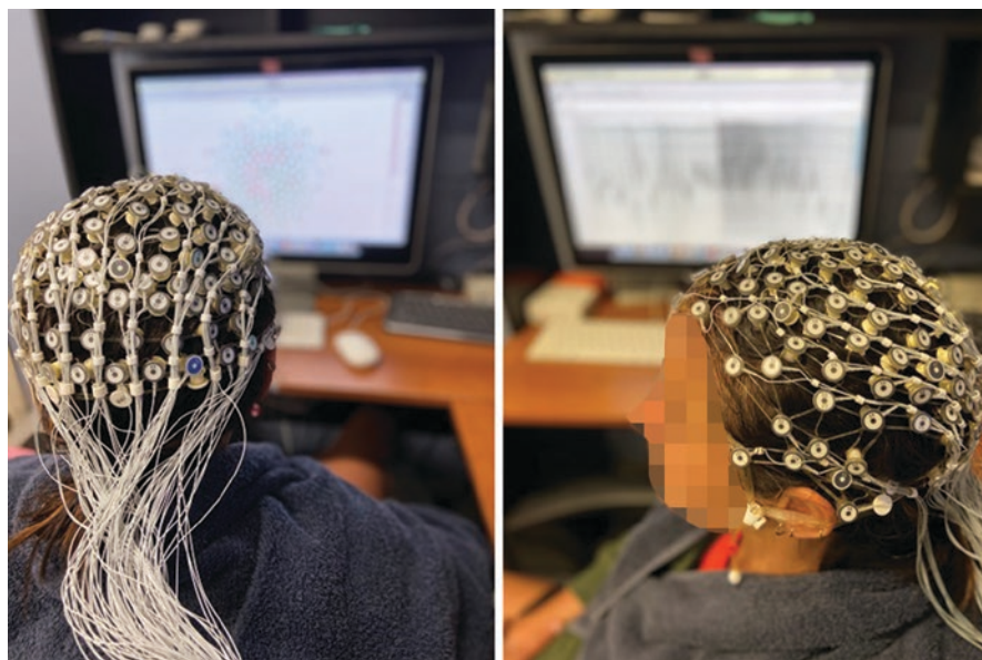
Fig. 4.1 128-electrode cap applied during routine EEG recording
