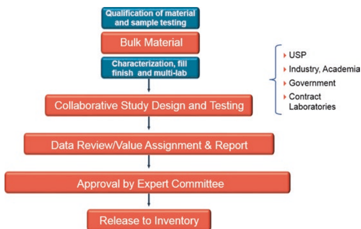
Fig. 2 Reference standard development process and collaboration with external laboratories
