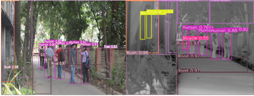
Fig. 5. Object detected on RGB and Thermal Images from test set. Non-maximal Suppression = 0.5, Confidence Threshold = 0.4, IoU = 0.5
