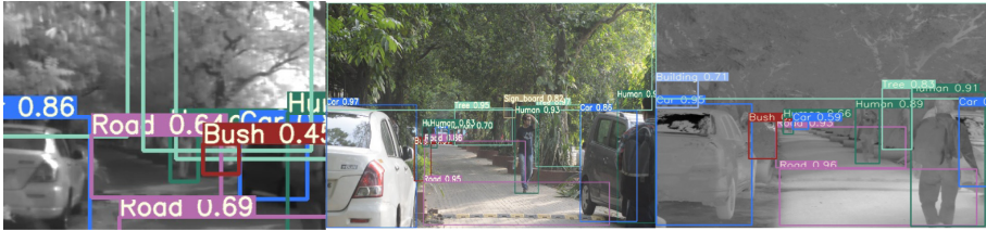
Fig. 6. Object detected on NIR, RGB and THERMAL Images respectively from test set. Non-maximal Suppression = 0.5, Confidence Threshold = 0.4, IoU = 0.5
