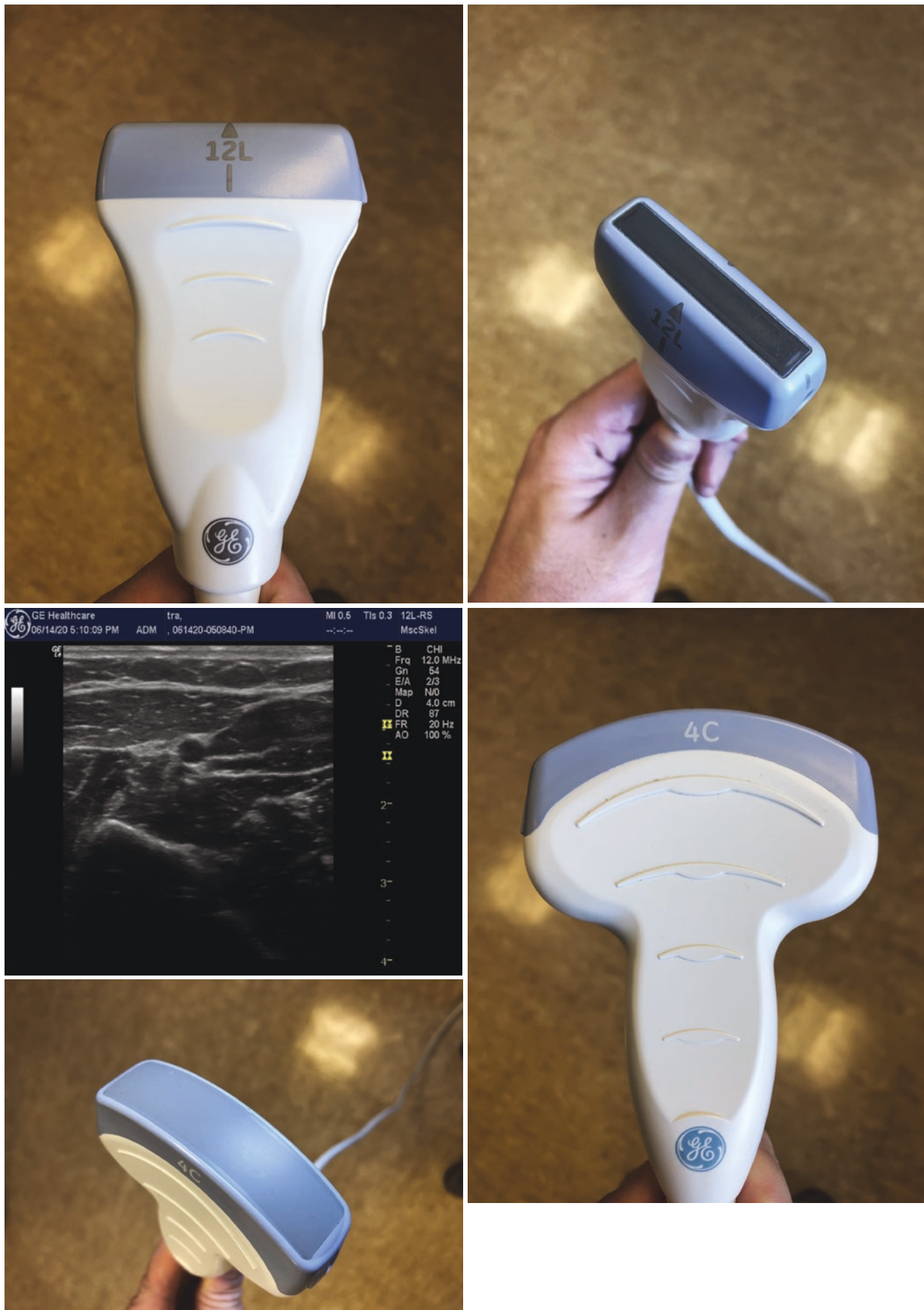
Fig. 10.4 Linear transducer (a) with view of footprint along with accompanying field of vision of a left forearm. Curvilinear transducer (b) with view of footprint along with accompanying field of vision of a left forearm
