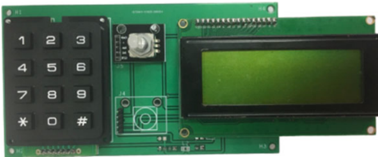
Fig. 6 The result product of the control panel board
