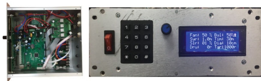
Fig. 13 Final fume hood control product
