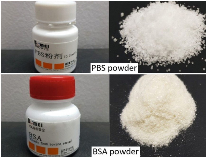
Fig. 1 PBS and BSA powders were used for preparing the lubricant of 25 mg/ml BSA
