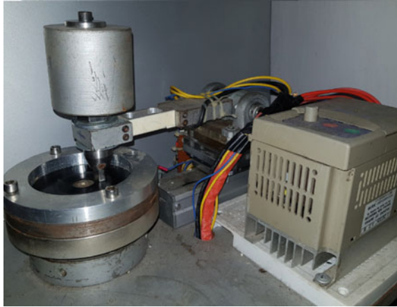
Fig. 2 A frictional testing apparatus was carried out for the measurement of COF
