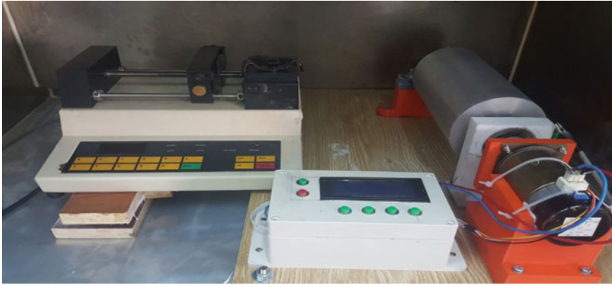
Fig. 4 The drum collector system
