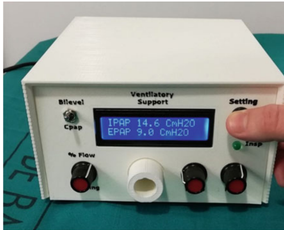
Fig. 2 Front panel of the ventilator. The Bilevel/CPAP switch allows selecting the type of pressure support: Bilevel pressure ventilation or continuous positive airway pressure, respectively. 'P-exp', 'P-ins': turning these knobs, while pushing button 'Setting', allows setting expiratory and inspiratory pressure, respectively. Green led on during inspiration. '%Flow' cycling: Turning the knob allows to set the % of maximum inspiratory flow threshold at which the device cycles to start expiration
