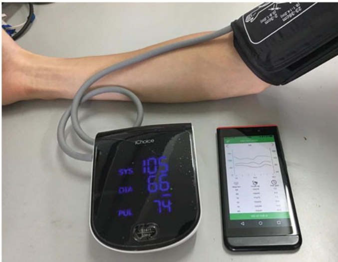
Fig. 5 The holter NIBP system with iChoice device and smartphone
