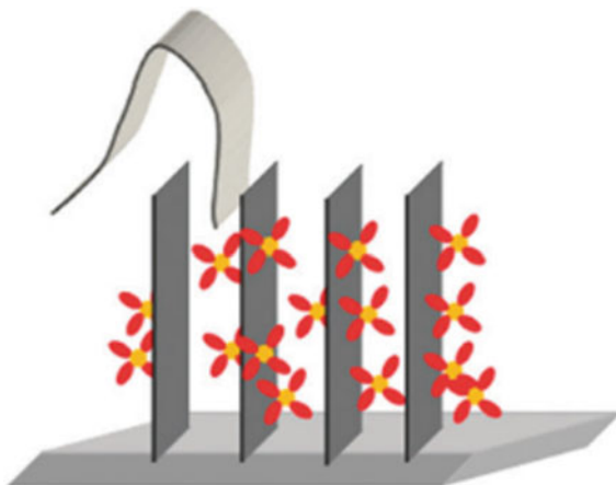
Fig. 5 Strategy for novel electrode structure: bimetallic nanodendrite hybrid catalyzed graphene sheets can be covered by a thin proton ionomer film and assembled on the proton electrolyte membrane. (Reproduced with permission from ref [86]. Copyright© the Owner Societies 2011)
