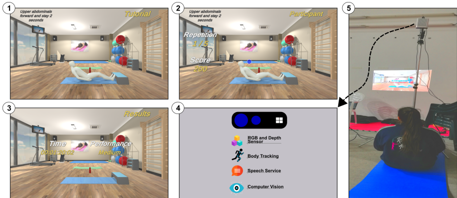
Fig. 4. Rehabilitation system in action. (1) tutorial view. (2) Participation view. (3) Result view. (4) Features of the Azure Kinect DK™ device. (5) User using the system [9].
