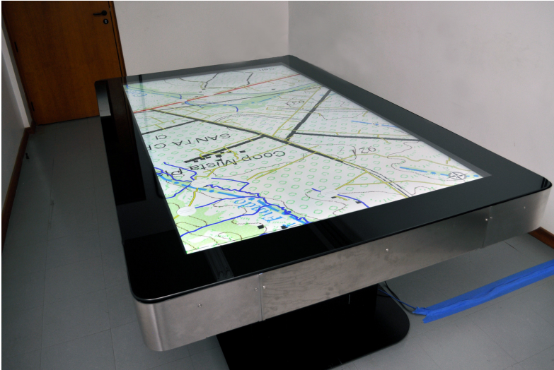
Fig. 2. Tabletop virtual tactical simulator [7].
