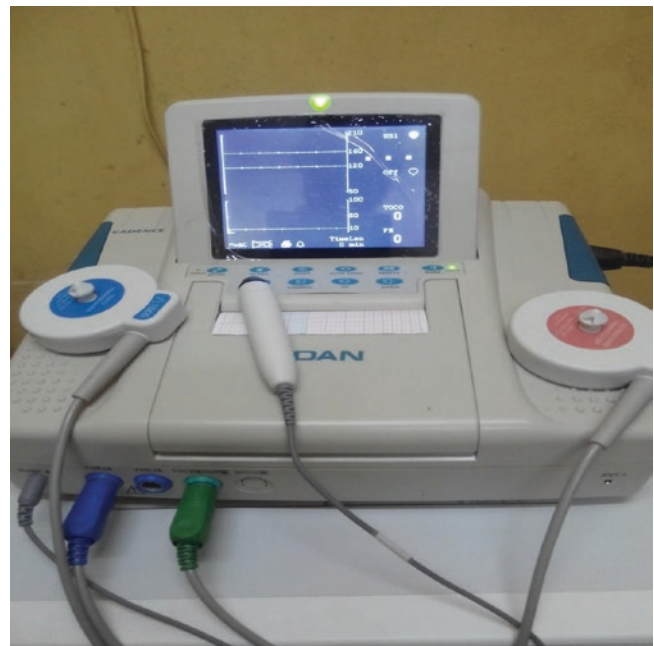
Picture of CTG machine (the cardiotocograph) with the Doppler probe, the event marker and the tocodynamometer (from left to right of picture)
