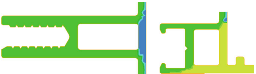
Fig. 5 Material streams in samples #1 and #2. The material from different streams is shown by different colors. (Color figure online)
