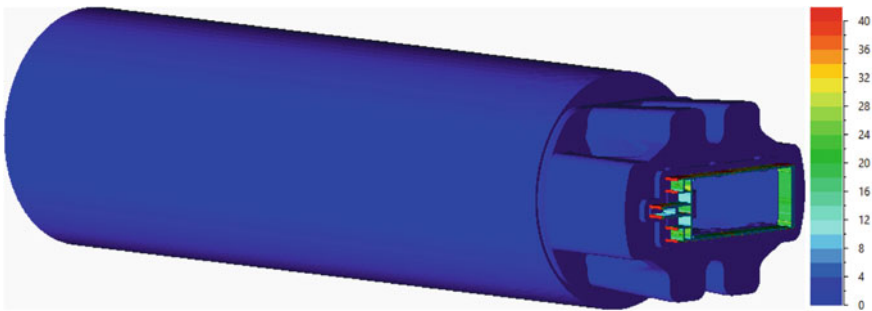
Fig. 2 Workpiece during extrusion simulation with strain field shown (the die set and container are not shown). (Color figure online)
