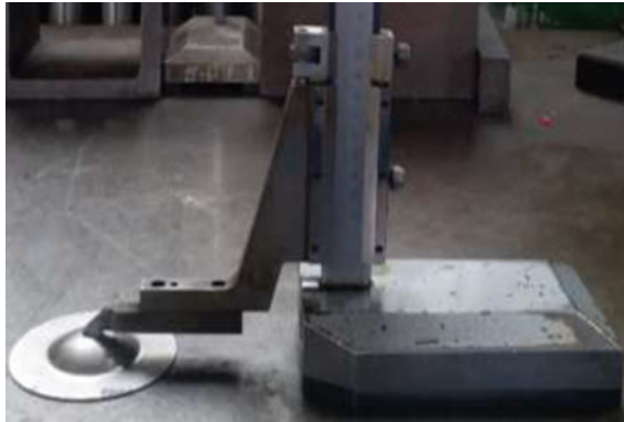
Fig. 8 The measurement tool used to measure the bulge height of each test specimen. (Color figure online)
