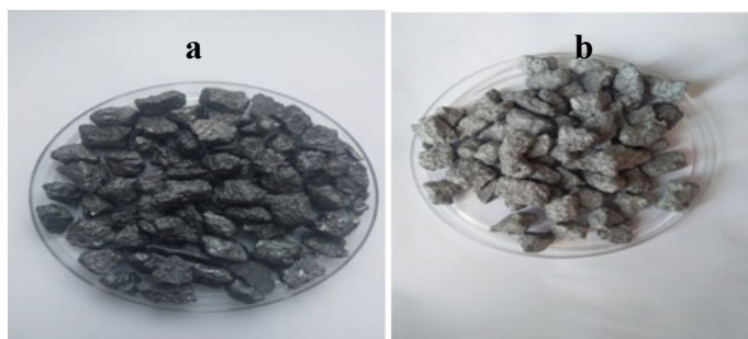
Fig. 15.1. Photographic image of GT-NTiO 2 a Before coating b After coating
