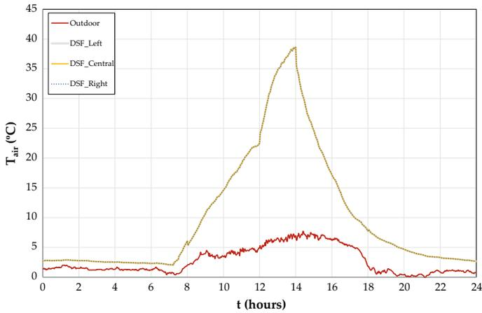
**Fig. 1.5** Evolution of DSF system indoor air temperature and of outdoor air temperature
