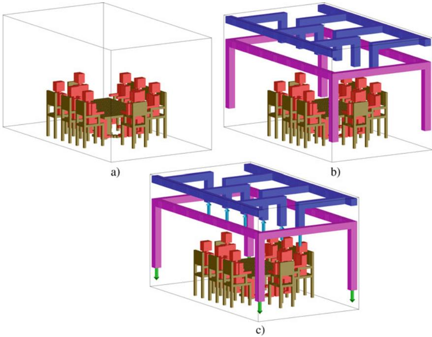
**Fig. 1.1** Numerical methodology used in the CFD model grid generation: **a** Representation of eight occupants, a table and eight chairs. **b** Including the inlet ventilation and the outlet system. **c** With inlet (light green arrows) and outlet (light blue arrows) airflow used
