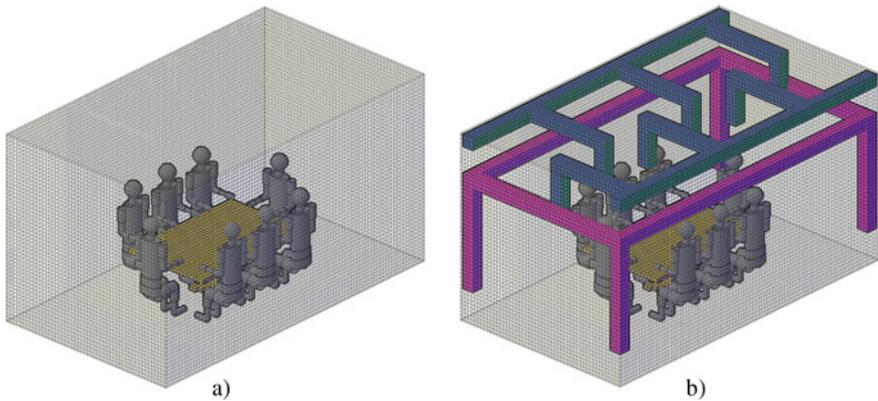
**Fig. 1.2** Numerical methodology used in the grid generation of the HTR model: **a** Representation of eight occupants, a table and eight chairs. **b** Including the impinging jets ventilation
