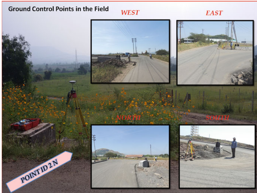
Fig. 19.3 Measuring ground control points in the field using dGPS
