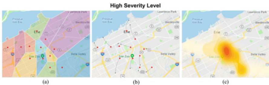
Fig. 8 Optimal allocation of 12 agents for the high severity level. (a) Optimal locations; (b) Routes from random starting locations to the optimal locations; (c) Crime distribution of high severity level
