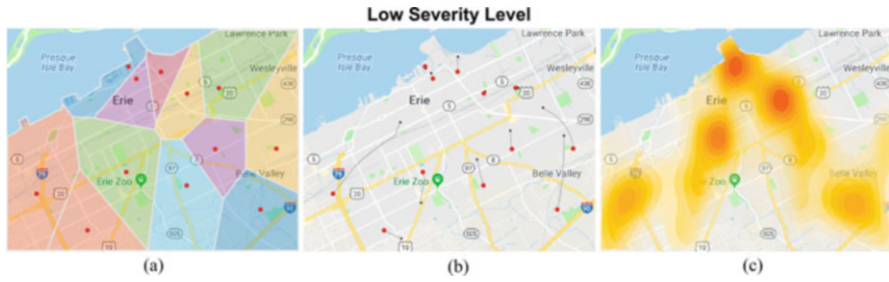
Fig. 6 Optimal allocation of 12 agents for the low severity level. (a) Optimal locations; (b) Routes from random starting locations to the optimal locations; (c) Crime distribution of low severity level
