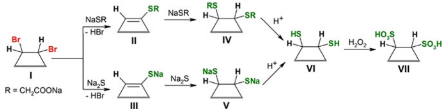
Fig. 13 Schematic of the sulfonation pathways starting from the brominated carbon surface
