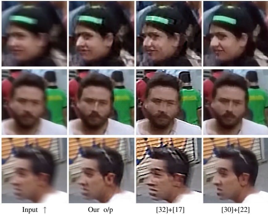
Fig. 6.7 Results on Gopro dataset [30]. Faces were cropped from the blurred images provided in the test set. Even though our network was not trained for such a real dataset, it was able to produce comparable results to the work in [30] that was specifically trained on Gopro
