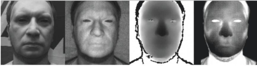
Fig. 13.2 Preprocessed images from a rigid mask attack; channels showed are grayscale, infrared, depth, and thermal, respectively. Channels were preprocessed with face detection, alignment, and normalization
