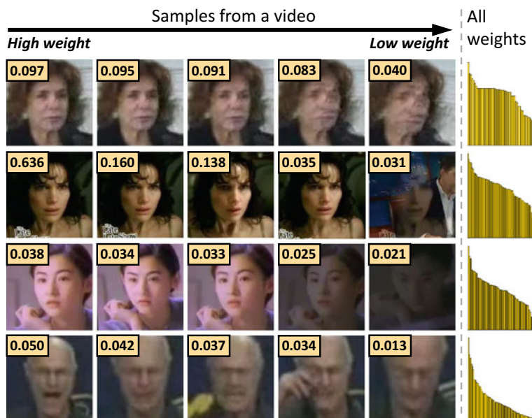
Fig. 10.7 Typical examples on the YTF dataset showing the weights of the video frames computed by NAN. In each row, five frames are sampled from a video and sorted based on their weights (numbers in the rectangles); the rightmost bar chart shows the sorted weights of all the frames (heights scaled)
