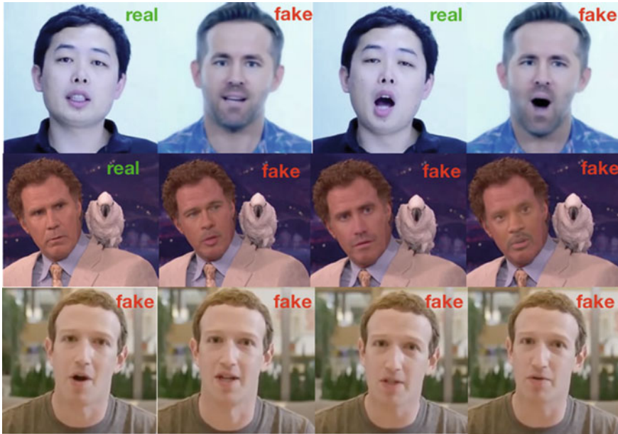
Fig. 12.1 Examples of AI-synthesized impersonation videos (DeepFakes). (top) Head puppetry entails synthesizing a video of a target person’s head using a video of a source person’s head, so the synthesized target appears to behave the same way as the source. (middle) Face swapping (DeepFake) involves generating a video of the target with the faces replaced by synthesized faces of the source while keeping the same facial expressions. (bottom) Lip syncing is to create a falsified video by only manipulating the lip region
