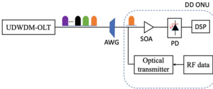
Fig. 7.16 A block diagram of DD-based ONU for UDWDM-PON
