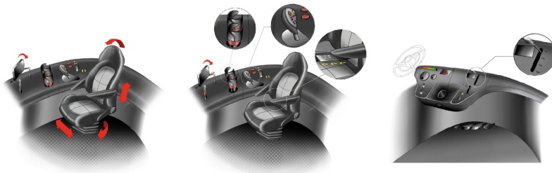
Fig. 1. General views of the design proposal for the tractor's cabin interior with ergonomics adjustment in the driver's seat, multi-purpose accessory, joystick and frontal panel.
