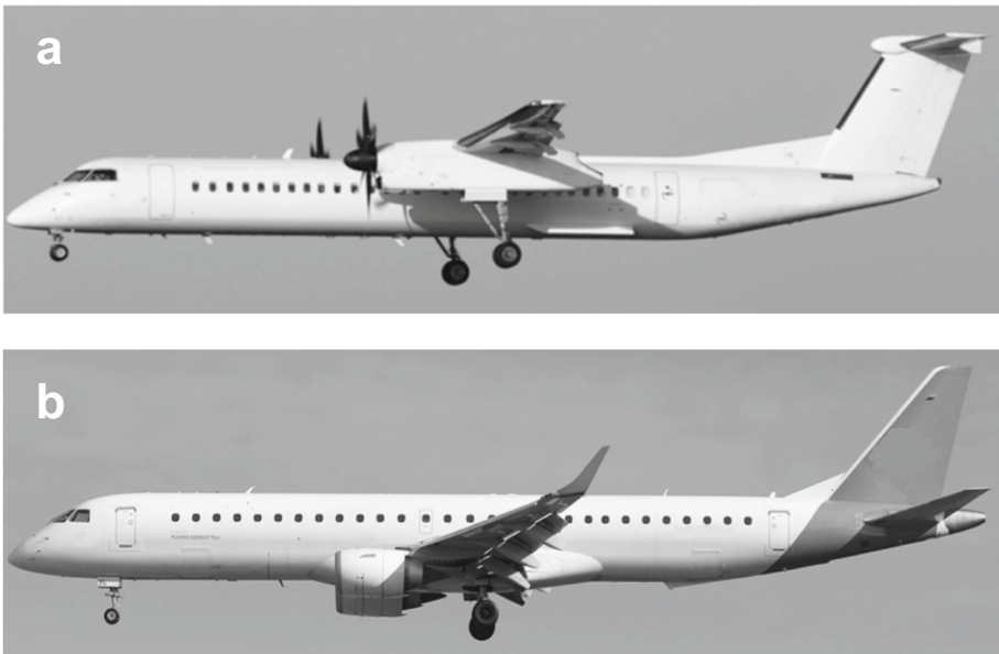
Fig. 1. Images of a turboprop aircraft (a) and turbojet aircraft (b) presented in Sects. 1 and 2 of the focus groups. Images were anonymized and presented in black and white.
