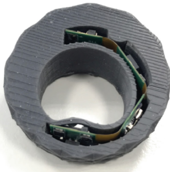
Fig. 2. Detail of the flexible electronic board inserted in the ring cover.
