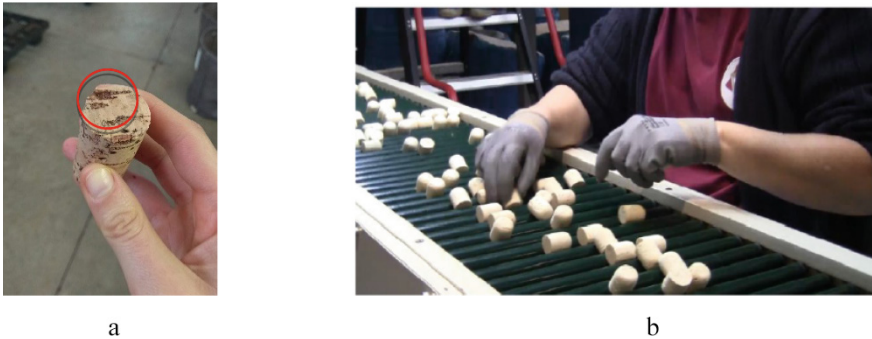
Fig. 1 a. Defective stopper. b. Manual selection of stoppers.
