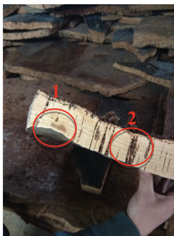
Fig. 2. Cork plank with some defects: 1 designated as verdura (“greenness”, which is a defect visible by the superficial accumulation of water in cork plank); and 2 as prego (“woody”, which is characterized by the presence of sharp nodes in the belly of cork planks).
