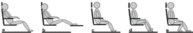
Fig. 6. Significant postures for sleeping (a and b), relaxing (a) and watching (c/d/e): studied by (Groenesteijn et al. 2014)
