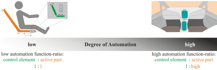
Fig. 1. Illustration of the degree of automation using the example of an electrical seat adjustment (left) and an autonomous vehicle cockpit (right)
