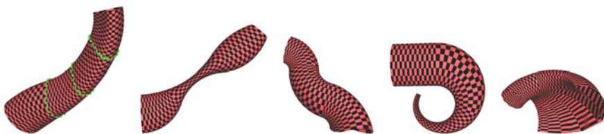
Fig. 15 Various deformations of a series of cylinders across multiple lattice volumes. On the left-most image we see in green the points that are inverse mapped in order to connect the series of volumes.
