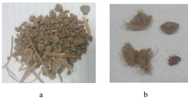
Fig. 6 Aggregates of plaster and mortar samples from house 02 in Saraylı a crushed brick particles, b cloth pieces and nut shells
