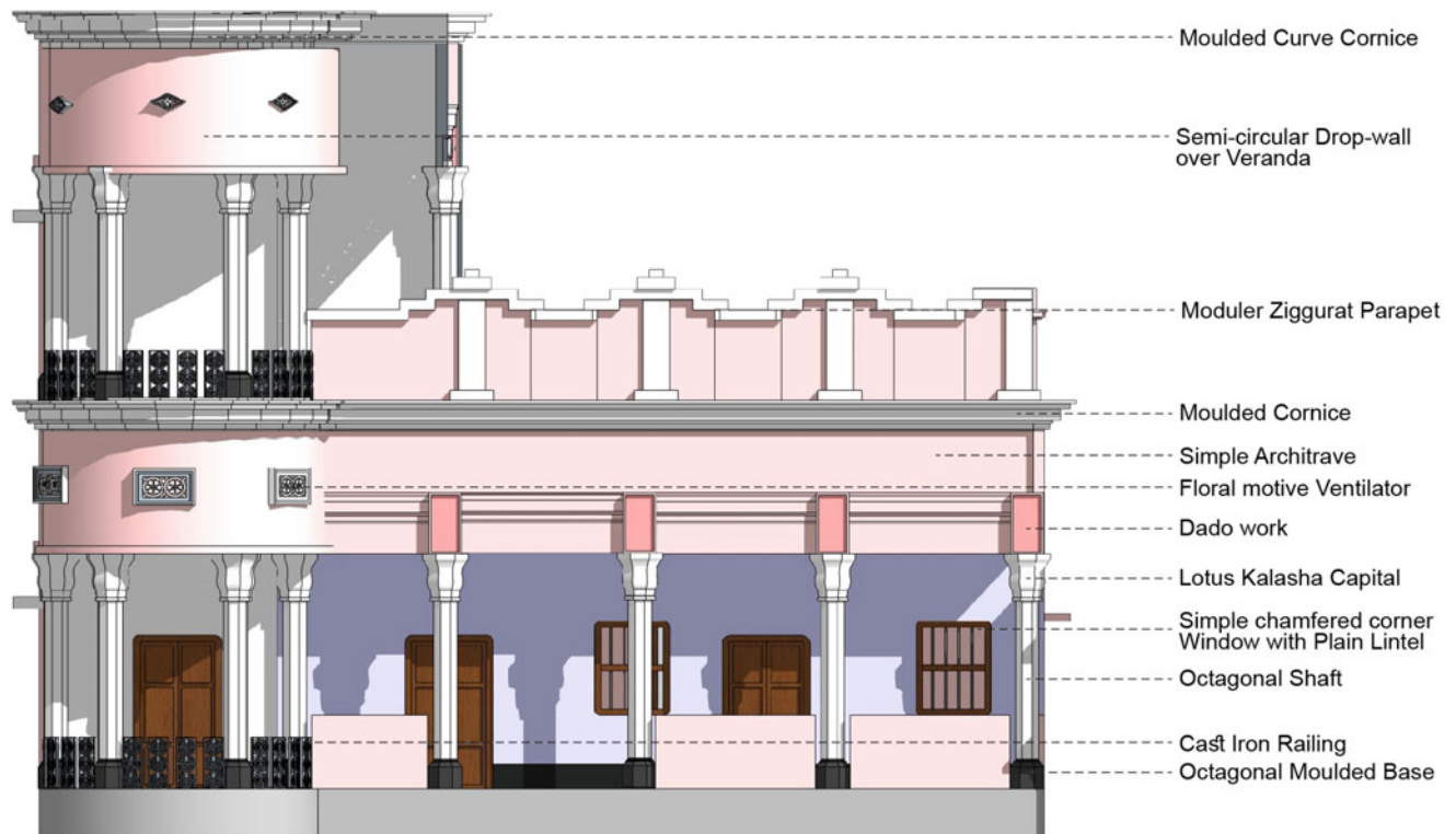
Fig. 14 Sakhina House (1950 AD) facade details (Source Drawn by Authors)
