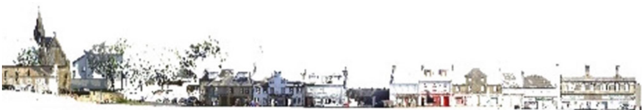
Fig. 11 Point cloud elevation of the street façade of conservation site including the church and site
