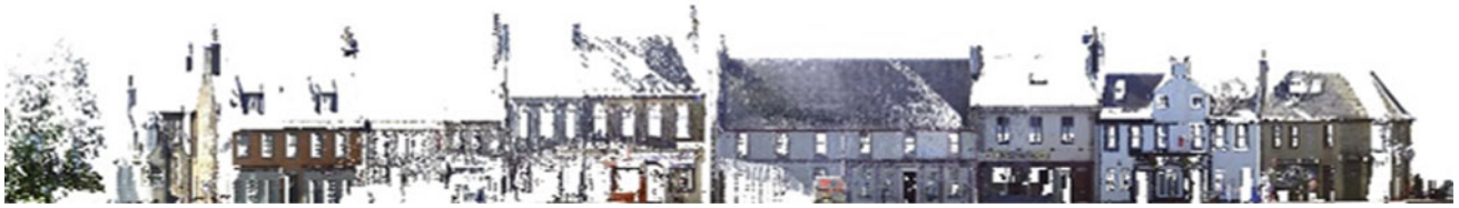
Fig. 12 Point cloud elevation of the street façade of the conservation area
