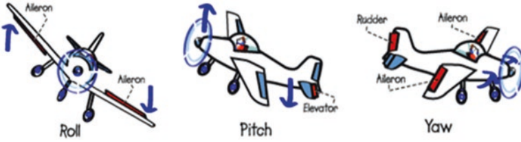
Fig. 3.2 Pitch, roll, and yaw in an aircraft (NASA official: Tom Benson)
