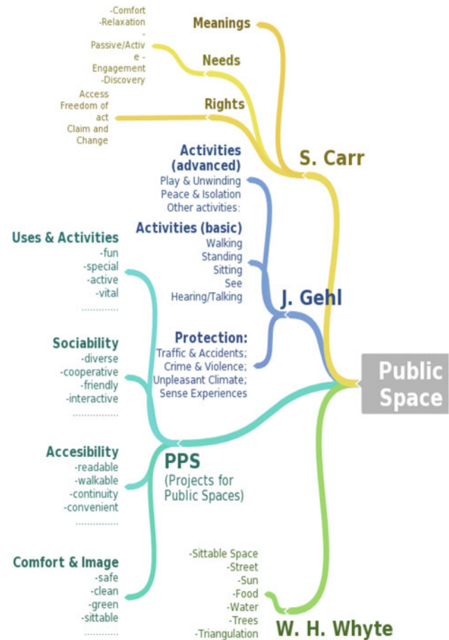
Fig. 5 Successful public space basic criteria. Source J. Gehl, S. Carr, PPS, and W. H. Whyte
