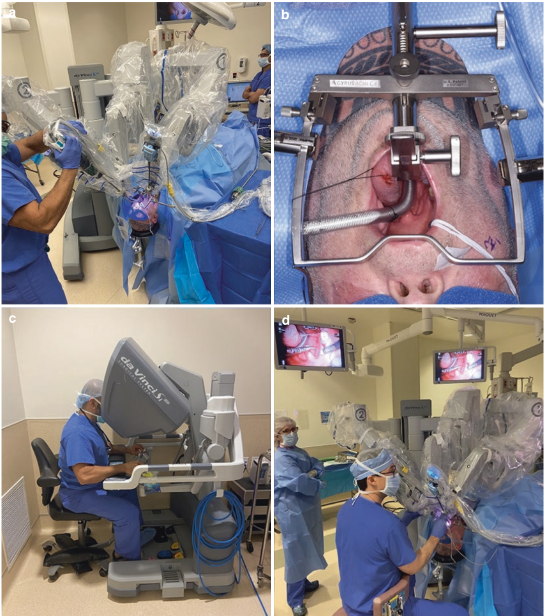
Fig. 15.3 (a) Positioning the robotic arms of the da Vinci Si system. (b) FK-WO retractor in position for view of the oropharynx. (c) Surgeon console in use. (d) Assistant at the head retracting and suctioning as needed
