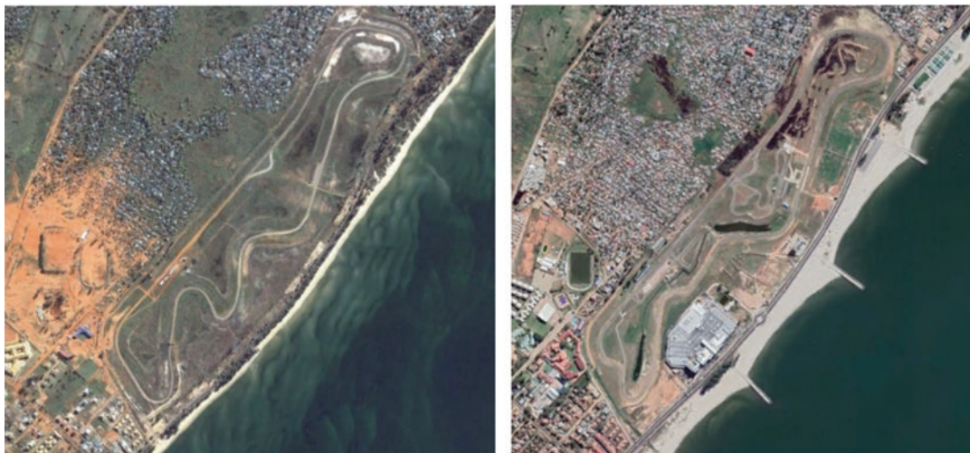
Fig. 18.3 Section of Maputo city Avenida Marginal (coastal line). (a) Without groyne (sea-break) and (b) with groyne allowing sand accretion up to 130 m into the sea
