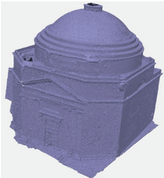
Fig. 6 Meshing - 2,075,610 faces and 1,044,046 vertices
