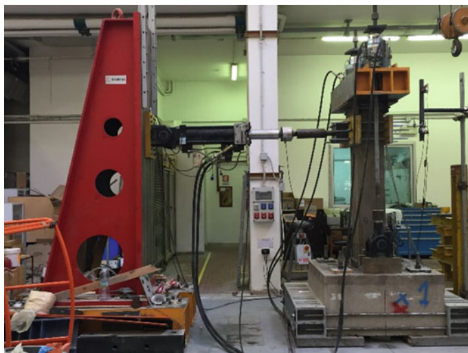
Fig. 4 Experimental setup for the cyclic pushover tests
