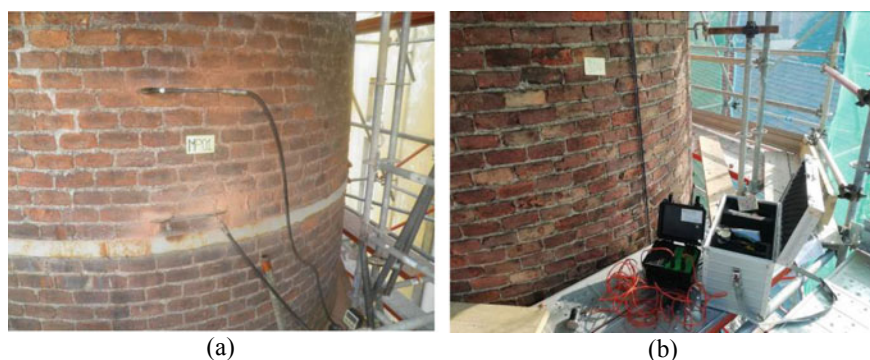
Fig. 4 Material characterization of masonry structure: a flat-jack and b sonic test position
