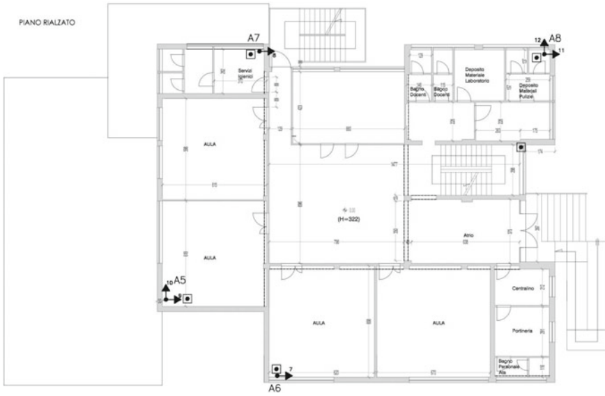
Fig. 4 Position of accelerometers placed at ground level
