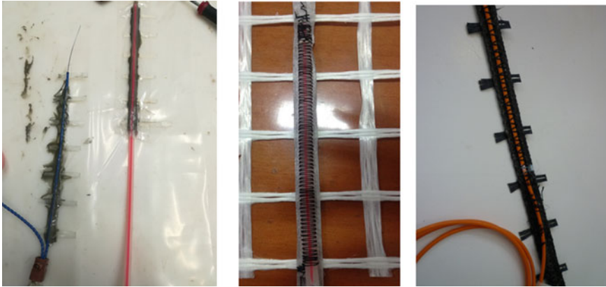
Fig. 1 Tested solutions for sensor-textile integration: gluing (left), stitching (center), weaving (right)
