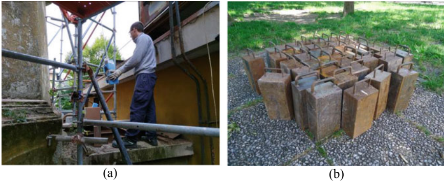
Fig. 7 a Drop weight input test and b masses of 25 kg
