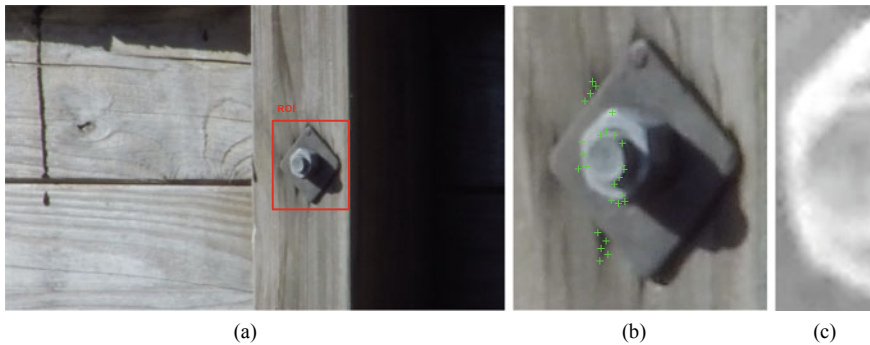
Fig. 5 Image processing: a reference frame with a selected ROI, b features for the feature matching technique, and c template for template matching technique
