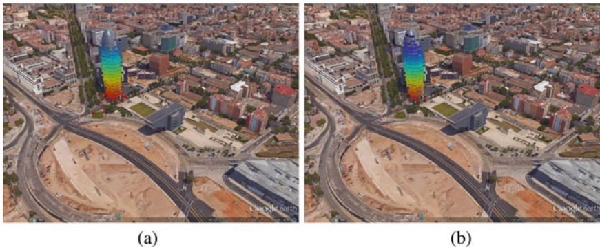
Fig. 4 Detected scatterers relocated on optical image without (a) and with considering the effect of thermal dilation (b)
