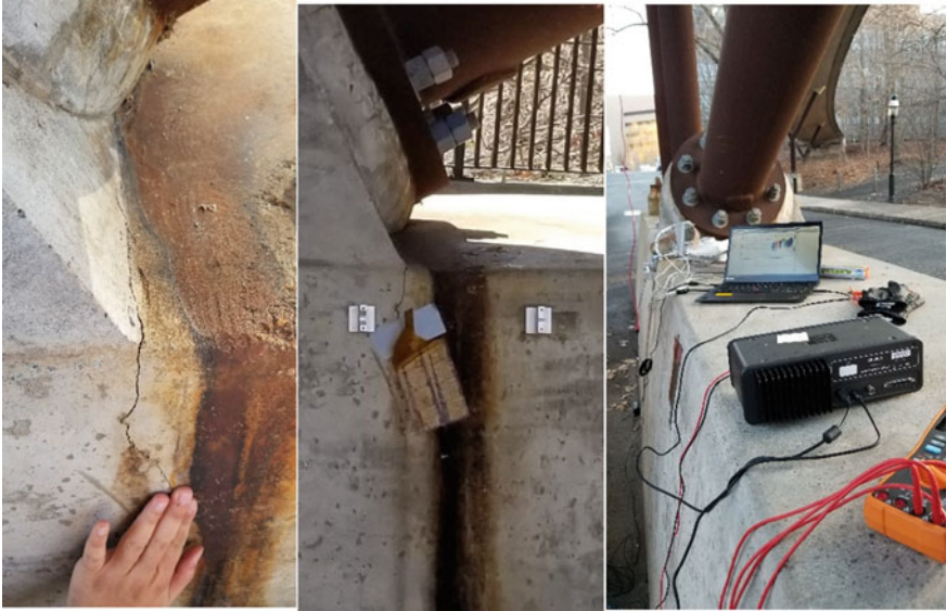
Fig. 4 The pre-existing shrinkage crack on the foundation (left), the sensing sheet glued to the crack (center), the setup of field experiment (right)
