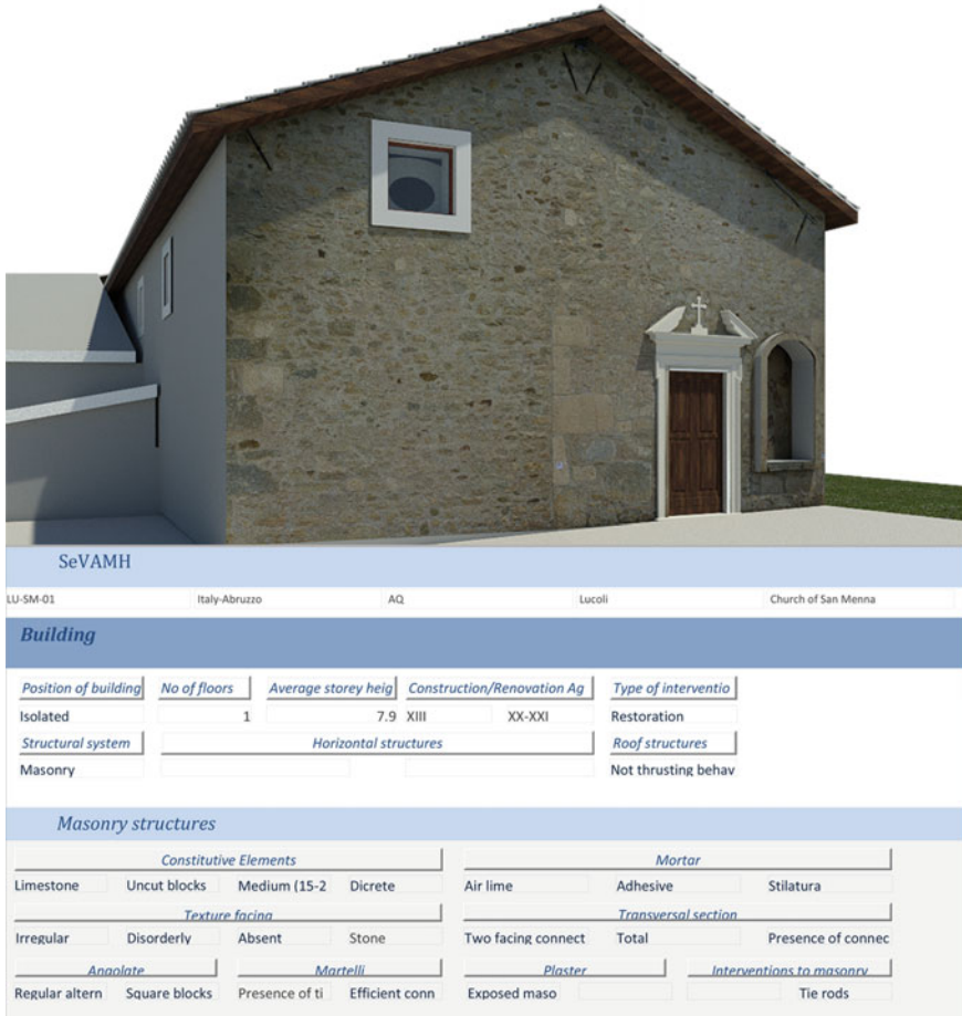
Fig. 4 Correlation between the parametric model and the building module of the SeVAMH form
