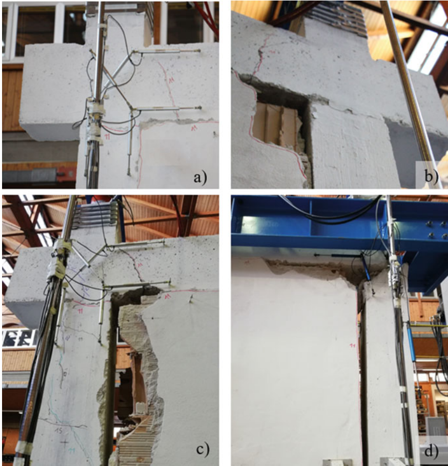
Fig. 4 Final damage state: a left side and b right side of the frame
