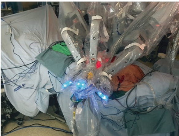
Fig. 3.4 Robotic arm positioning for the da Vinci. The patient cart is stationed ipsilateral to the rectus being dissected and perpendicular to the patient. The camera arm is flexed 90° at the elbow. Maximizing distance between patient clearance joints is essential. Instrument arm elbows are placed akimbo to the camera arm to minimize interference. Ports are placed contralateral to the rectus being harvested
