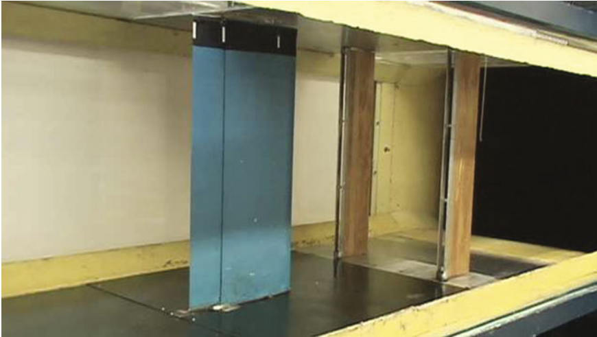
Fig. 6 Photograph of the experimental model with gust generator in the wind tunnel test
