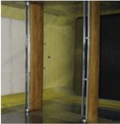
(a) Photograph of gust generator
