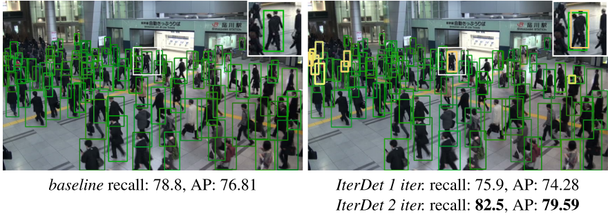
Fig. 1. The results of original Faster RCNN (left) and the proposed IterDet based on Faster RCNN (right) for the same image from CrowdHuman test set with visible-body annotations. The boxes found on the first and second iteration are marked in green and yellow, respectively. The metrics for baseline and IterDet after the first and the second iterations are listed below the images. (Color figure online)
