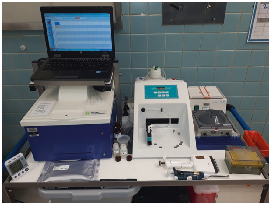
Fig. 16.3 The Future Diagnostics the point-of-care intraoperative parathyroid hormone assay which is a mobile system that is deployed to the appropriate operating room. The setup at our institution is demonstrated
