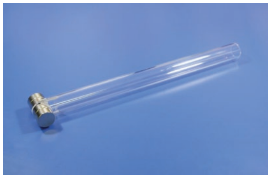
Fig. 16.18 Photograph showing the apparatus used for extracorporeal magnetic guidance. Four neodymium magnets (20 mm in diameter, 10 mm in thickness, 8000 gauss in total) are attached at the head of the handle. This apparatus is used to move or hold the magnet in the bowel loops
