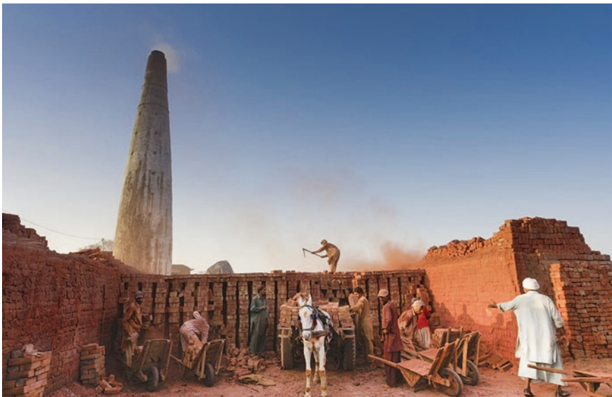
Fig. 52.1 A typical Bull's trench brick kiln from Pakistan
