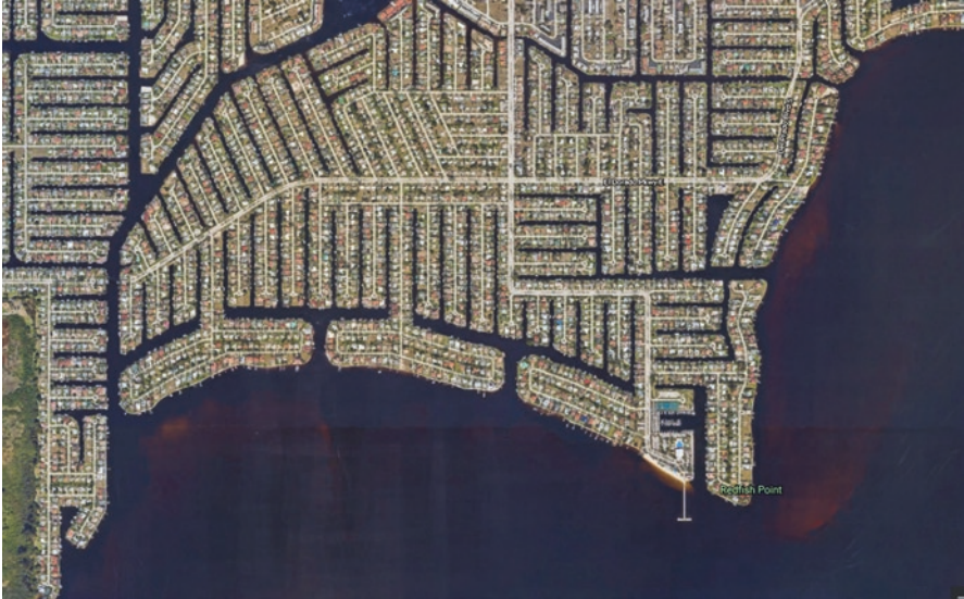
Fig. 12.8 Aerial view of high density of low-lying homes along canals in southern Cape Coral. These canals, created by dredge and fill, provide access to the Caloosahatchee River and the Gulf of Mexico for hundreds or even thousands of homeowners. (Source: www.earth.google.com , accessed 6/25/2020)
