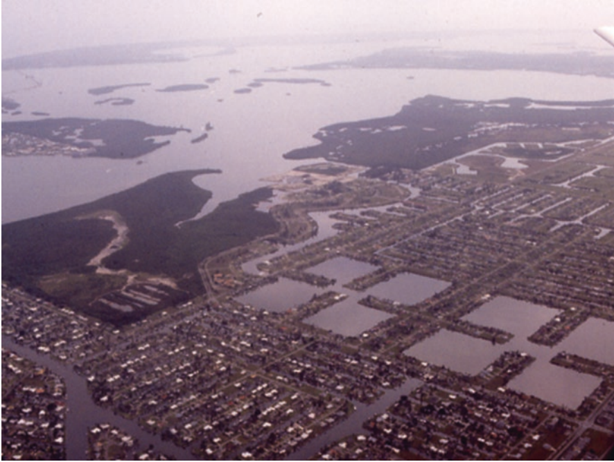
Fig. 12.4 Aerial view of the eight-lake region in the southern portion of Cape Coral. These lakes were excavated during dredge and fill operations to provide fill for home sites. Coastal wetlands and Sanibel Island are visible in the background. (Source: Photo taken by the author)
