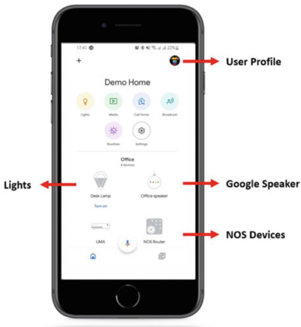
Fig. 8.9 Google Home App with lights, NOS network router and STB, with voice integration
