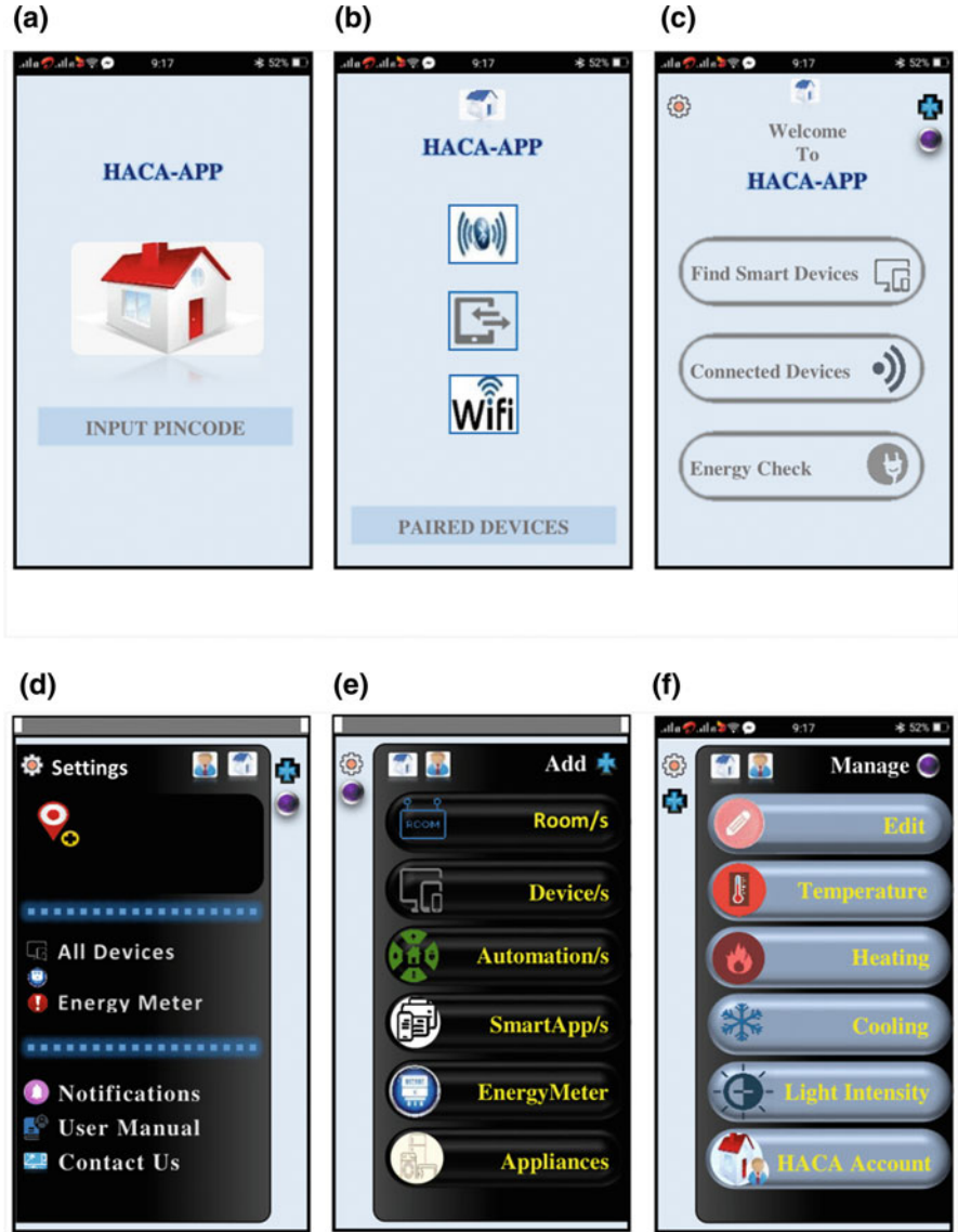
Fig. 19.4 (a) Specify password, login HACA-App; (b) paired with cell data/Bluetooth connectivity/Wi-Fi link; (c) welcome to HACA-App, Select options ; (d) select Settings: add locations, check connected appliances, notifications, update HACA-App, etc.; (e) select Add: add rooms, appliances, devices, energy meter, etc.; (f) select Manage/Edit: manage HACA account, edit features, manage temperature, etc. HACA-App flowchart configuration of the proposed framework [screenshots]
