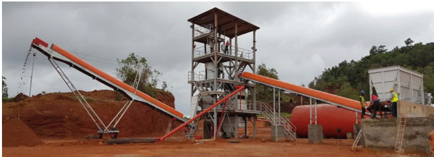
Fig. 5 Tailing beneficiation plant of SMHL, Sierra Leone
