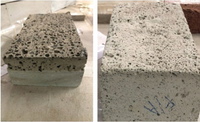
Fig. 5 Light weight foamed geo-polymer (Fly ash + GBFS)
