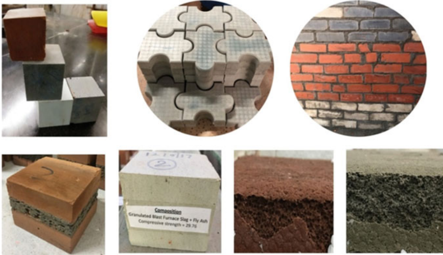
Fig. 4 Aluminosilicate (industry rejects) based geo-polymer products
