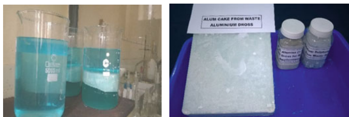
Fig. 5 Alum cake extracted from waste dross
