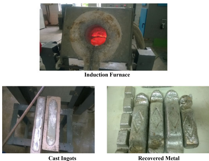
Fig. 3 Metal recovery processes from Aluminium dross
