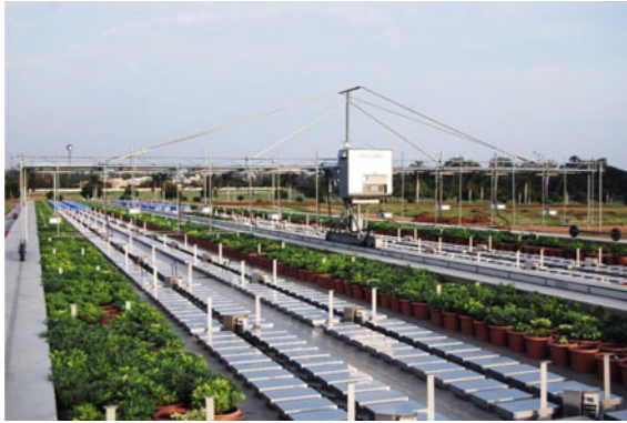
Fig. 11.4 Overview of the LeasyScan platform at ICRISAT. A groundnut crop is seen on side strips. The central strip shows the installation of load cells to allow the continuous weighing of the pots. Eight scanners (small white boxes) can be seen, attached to an irrigation boom that travels over the crop, on top of a center and two side walls. The central metal box has a key role to ensure a steady platform movement
