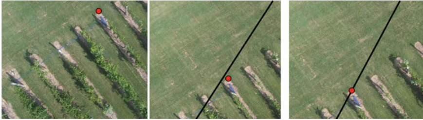
Fig. 4.5 Epipolar verification between two temporally distant frames that correspond to the same geolocation. Left: frame #56 with a red marked point. Middle: The corresponding epipolar line on frame #98 corresponding to the red marked point in the left frame (#32). Right: The same epipolar line but plotted after applying loop closure in the pose estimation. As one can see, the epipolar line passes through the ground truth point, in this case
