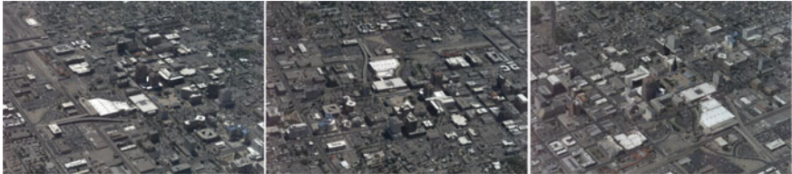
Fig. 4.7 A few sample frames in a high-altitude WAMI dataset corresponding to the downtown of Albuquerque, NM. The actual image frame sizes are 6600 \times 4400 pixels
