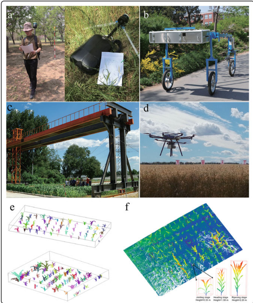
Fig. 6.3 Field phenotyping tools for crops: a mobile monitoring tool; b mobile monitoring vehicle; c unmanned ground vehicle (UGV); d unmanned aerial vehicle (UAV); e the individual segmented results of maize plant analysis from terrestrial lidar data using deep learning; f group data registered from six scanning stations for maize growth, and three representative maize plants of the three growth stages (jointing stage, heading stage, and ripening stage) are shown in the right corner. (Figure 6.3a–f are courtesy of Qinghua Guo, Chinese Academy of Sciences, China)
