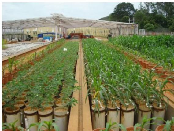
Fig. 11.3 Overview of the lysimetric platform at ICRIASAT (LysiField), showing the large tubes (25 cm diameter, 2.0 m length), which are set in trenches and allow a planting density of about 10 plant m^{-2} . A pigeon pea crop is seen on the left trench and a sorghum crop in the central trench
