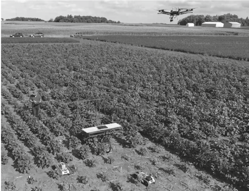
Fig. 7.1 Plant breeder taking field notes which can be complemented with, or independently collected using pushcart, ground robots, and an aerial system
