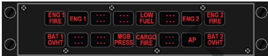
Fig. 4 Failure indication information display of EC175 helicopter
