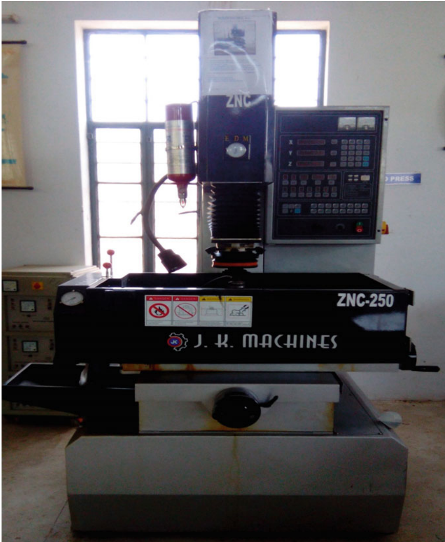
Fig. 15.3 ZNC 250 electric discharge machine
