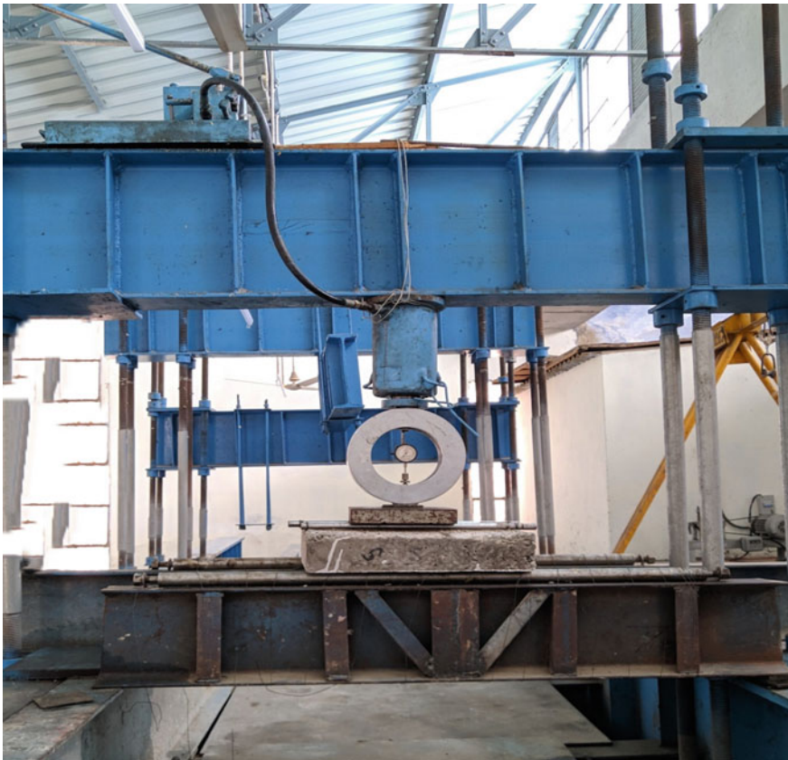
Fig. 19.3 Flexure testing of slab
