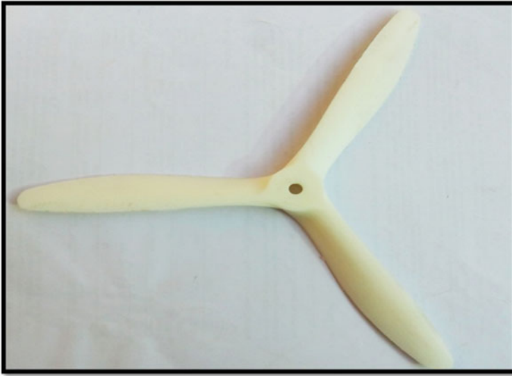
Fig. 5.6 New modified propeller having three rotors
