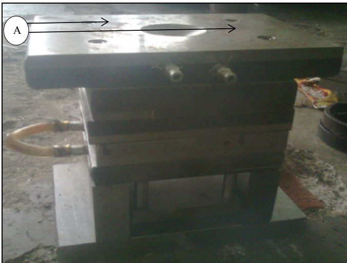
Fig. 47.2 A Indicate the high stress induced in die
