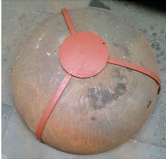
Fig. 12.7 Marking jig on the dish end
