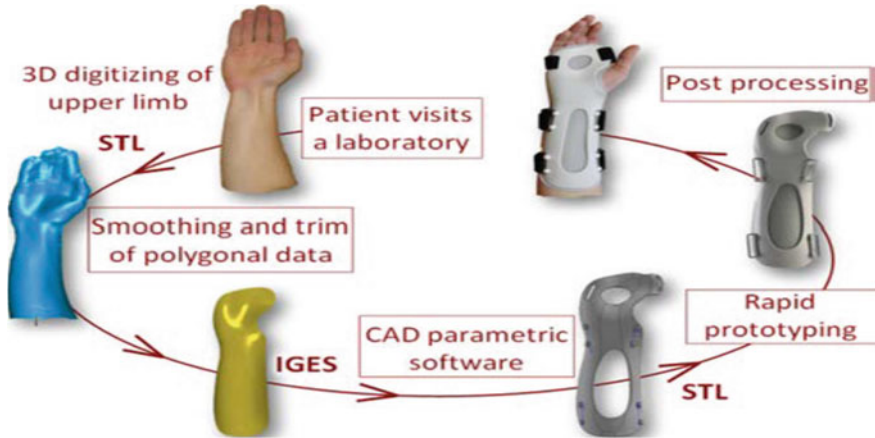
Fig. 22.6 Design process of the upper limb orthosis [11]
