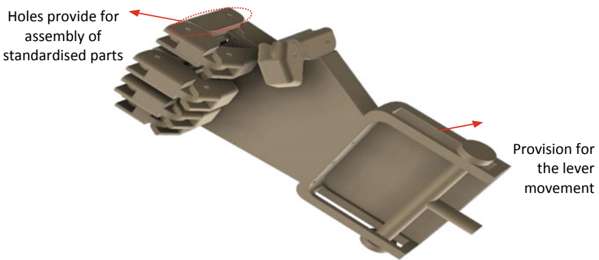
Fig. 20.3 A 3D view of the modeled prosthetic hand in closed fist position
