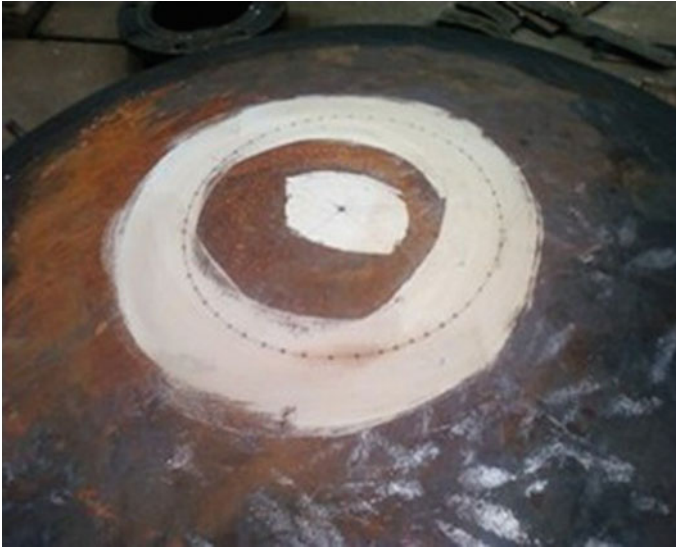
Fig. 12.4 Marking on the dish end
