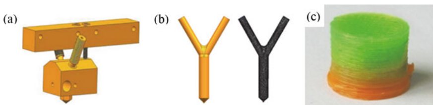
Fig. 44.4 a Assembly of entire model, b 3D model of flow channel and c 3D printed objects [17]
