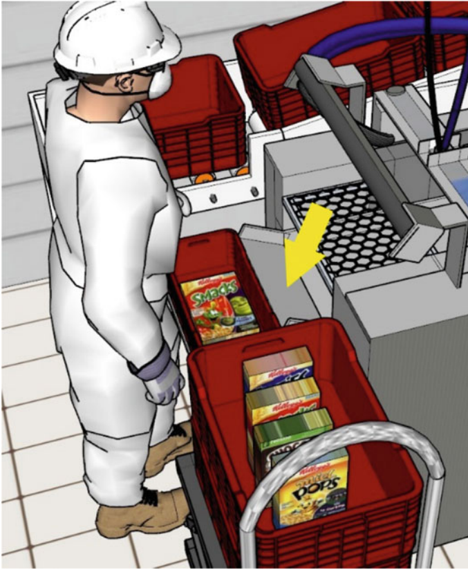
Fig. 12.10 Proposed modification of the work surface
