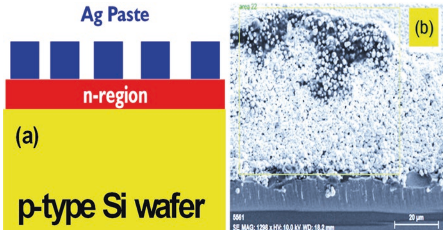
Fig. 4.53 Cross-sectional diagram of the screen-printed TLM pattern on an n-doped Si wafer used in this study (a) and low-resolution SEM image of screen-printed silver paste after drying (b)
