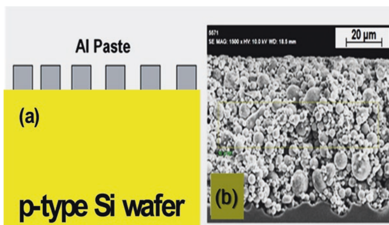
Fig. 4.40 Pictures of cross-sectional diagram of screen-printed TLM pattern on p-doped Si wafer (a) and low-resolution SEM image of screen-printed Al paste after drying at 100 \text{ }^\circ\text{C} for 10 min (b)
